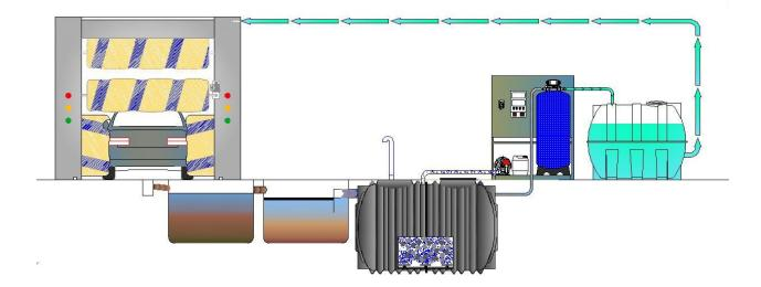
A complete line of carwash water treatment consists of a set of treatment operations, placed in series, with a view to achieving the predefined treatment objectives. In order to maximize water recovery and treatment, we recommend the following treatment line:
